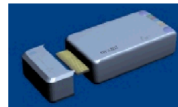
Figure 2. The i-WAND, a device that acts as a hub for the construction of pluggable body area networks.
