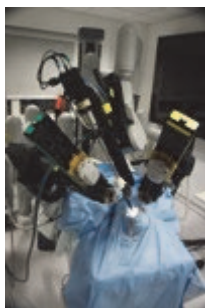
Fig. 2. Arrangement of the da Vinci endoscope and instrument arms in the left supraorbital subfrontal approach, demonstrating the difficulty in parallel insertion through a single keyhole craniotomy
