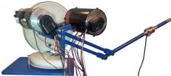
Fig. 3. Manufactured hybrid actuator system and actuator for 2 DoF system
