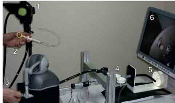
Fig. 1 Robotic control flexible endoscope: (1) Traditional endoscope with driving means for tip steering, (2) Manual instrument control (3) Multi-DOF controller for tip steering and shaft control, (4) Driving means for shaft actuation, (5) Training model, (6) Monitor.
