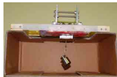
Fig. 2 MAGS test with handle on top, meat in middle, and one DOF module on bottom with weight attached.
