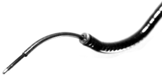
Fig. 3 Two-section concentric tube robot deployed through endoscope working channel. Distal section is monopolar cautery tool.
