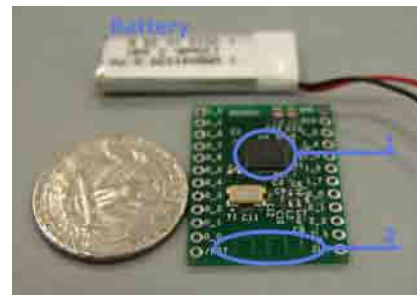
Fig. 4 Custom made PCB board with 1) CC2530 Zigbee transceiver; and 2) Chipcon AN043 antenna.
