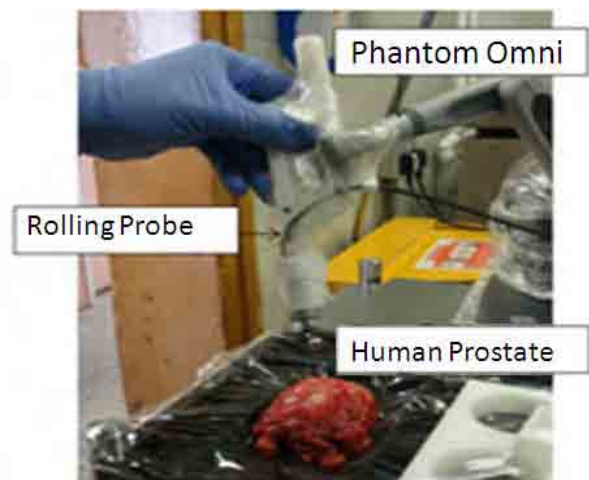
Fig. 2 Rolling indentation experiments conducted on human prostate.
