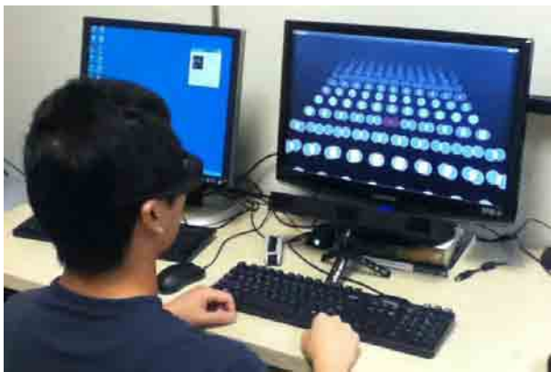
Fig. 1 Measuring gaze with a Mirametrix binocular eye tracker when viewing an active stereo display.
