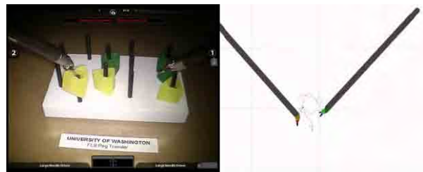
Fig. 3 (Left) View through the endoscope of a surgeon performing the FLS block transfer task. (Right) 3D rendering of the surgical tools and toolpath at the same moment based on a 3D model of the surgical tools and recorded position, orientation and end-effector pose data.
