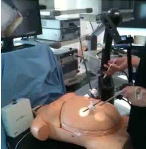
Fig. 2 Setup of the cadaveric porcine livers in the ELITE simulator with the SOLOASSIST device and ICSAD.
