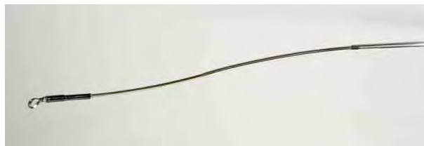
Fig. 1 A continuum robot made from three precurved elastic tubes. The robot is able to elongate and bend controllably as the tubes axially rotate and extend. A ring curette similar to those typically used in pituitary surgery is attached to the robot's tip.
