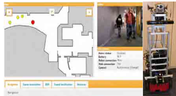
Fig. 3 The remote presence interface (left) and the uncovered health care robot (right).
