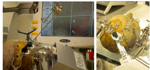
Fig. 4 Combined setup neuro-navigation (VectroVision, BrainLAB) and B-RobII during cadaver trial
