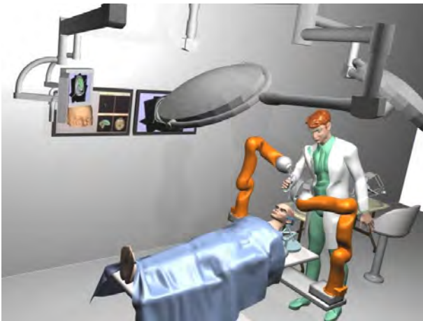
Fig. 1 The ACTIVE robotic system concept showing two manipulators being positioned by the surgeon under hands-on control. Also visible are the haptic master station, surgeon interface and workspace monitoring cameras [2].
