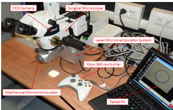
Fig. 1 Experimental setup: the new laser micromanipulator system is attached to surgical microscope. A real-time video from microscope camera is shown on laptop screen. Mechanical micromanipulator and Xbox 360 controller are shown.
