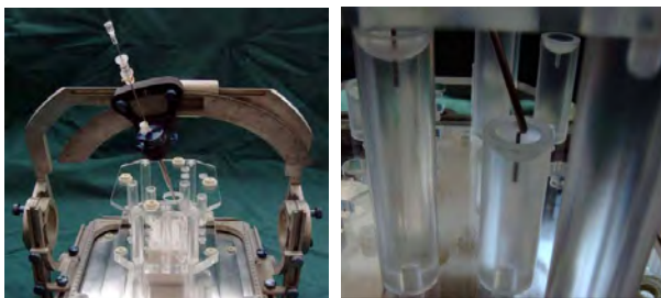
Fig. 3 Measurement setup for stereotactic frame and evaluation of targeting accuracy
