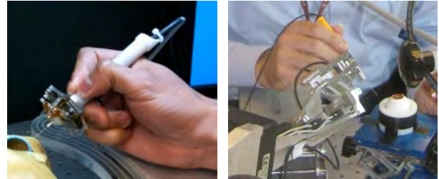
Fig. 5 (Left) CMU MICRON handheld robot; (Right) JHU cooperatively controlled Steady Hand robot
